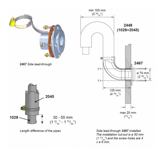
A side lead-through is installed in the side of the boat or in the transom. In sailboats it is recommended to install it in the transom. The installation always requires a so-called goose neck. Make the necessary installation cut-outs and spread a suitable sealing agent on both sides of the seal and on the screw holes. This will ensure that the connection is waterproof.
