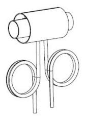
It is recommended that a drainage lock is installed if there is a risk of condensed or splash water entering the exhaust. If necessary, a drainage lock can be installed into the exhaust pipe of a hull lead-through, but note the drainage lock must be positioned after the gooseneck.
