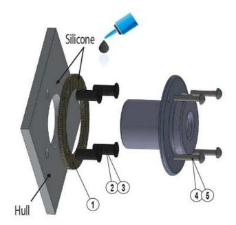
An insulation kit (**2461**) must be used to insulate the lead-through from the boats metal hull. The insulation kit insulates the exhaust gas lead-through and the device from each other. In fault situations the insulation kit prevents electric circuit running between the metal hull and the device. This could result the oxidation or malfunctioning of the devices circuit board and the circuit board would be damaged.
