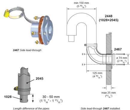
Side lead-through **2467** installed. The installation cut-out is  $\emptyset$  50 mm (1  $\frac{31}{32}$ ) and the screw holes are 4 x  $\emptyset$  6 mm.
